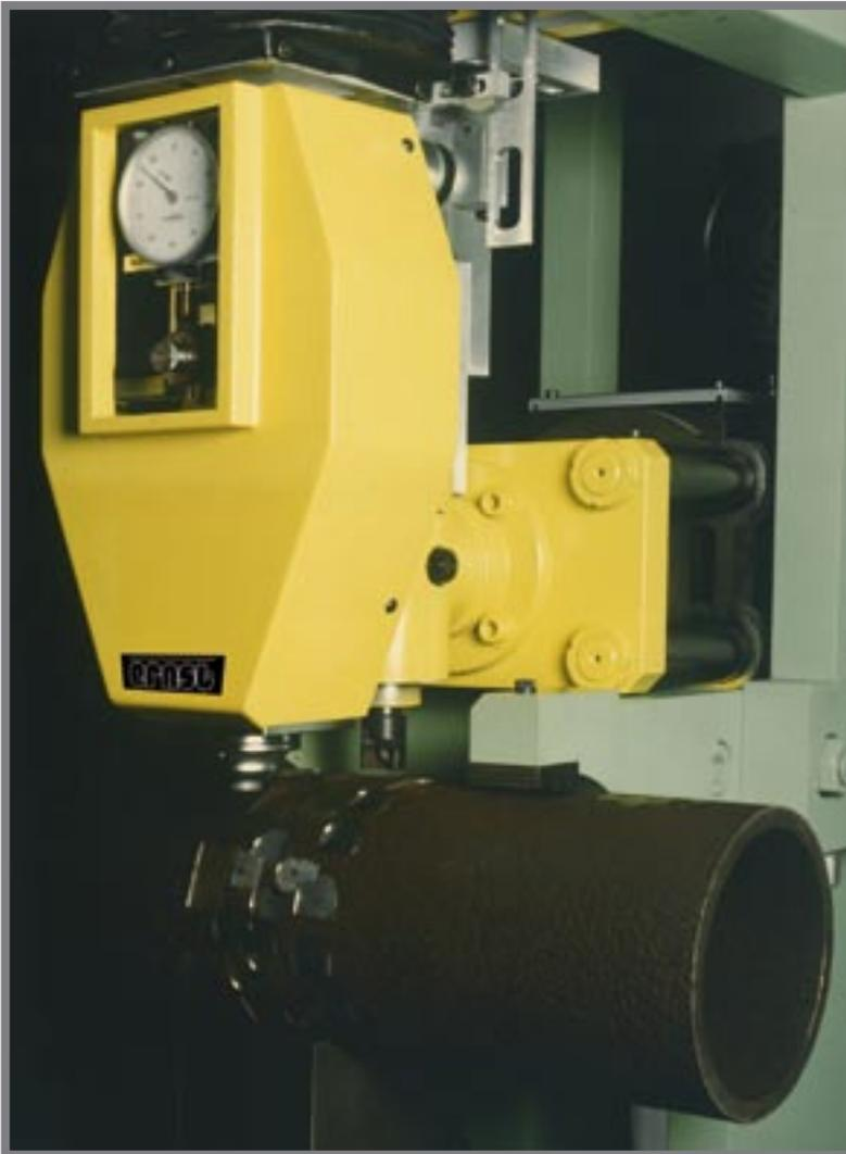
The BRE-AUT hardness tester tests the hardness based on the difference in penetration depth between preload and load, using loads and indenters requested for Brinell Standard testing. The results, after having been processed by a microprocessor, are shown on the display in Brinell values.
