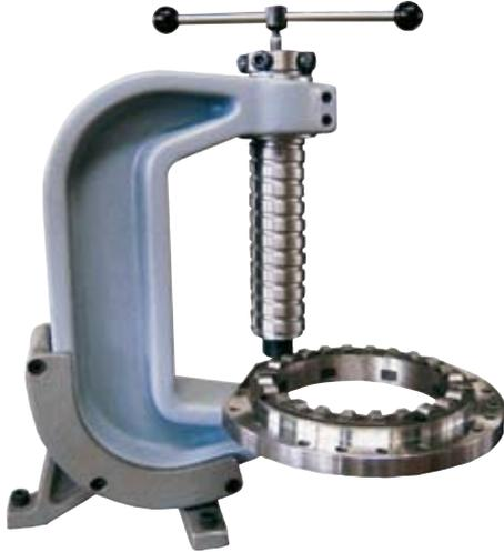
The static system allows load application via a lever on a clamp, particularly suitable for testing of castings. The screw system allows immediate load application.
