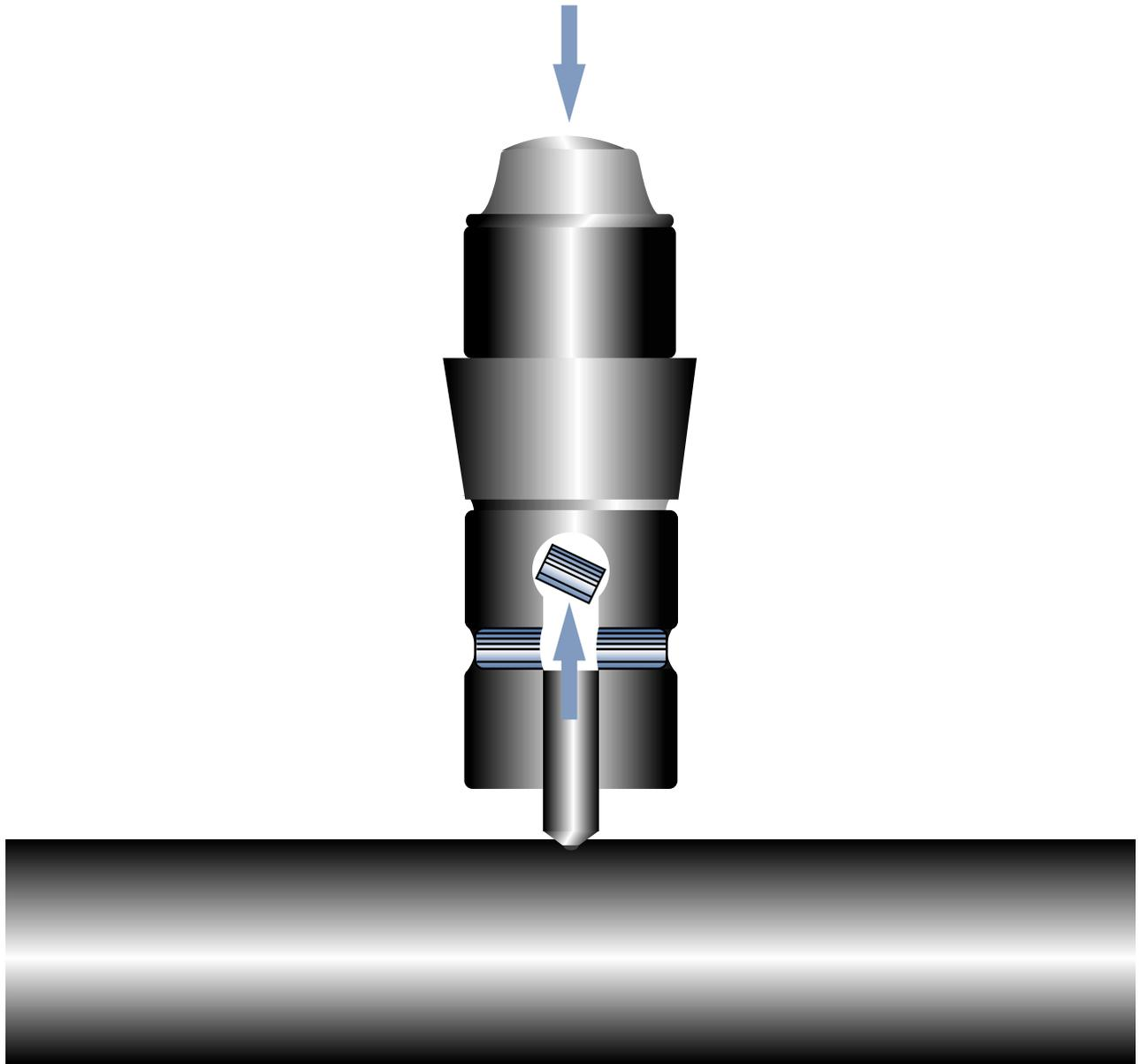
The ERNST calibrated pin system replaces the impact bar system giving a greater versatility and high accuracy. The indentations can be made very quickly even by an unskilled operator. The indentation can be read immediately, or at a later time by an inspector.
